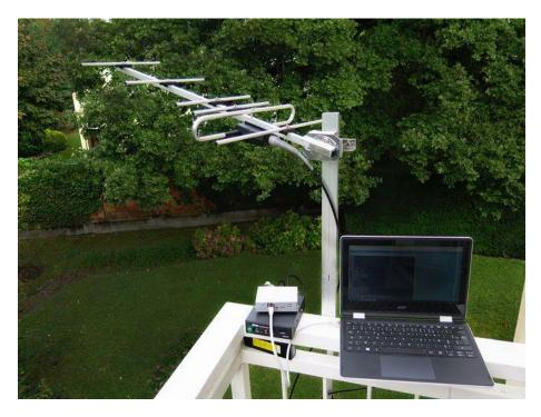
Data links work over the medium-range UHF band, but for the best results, a directional antenna is used.Photo: F4HDK
